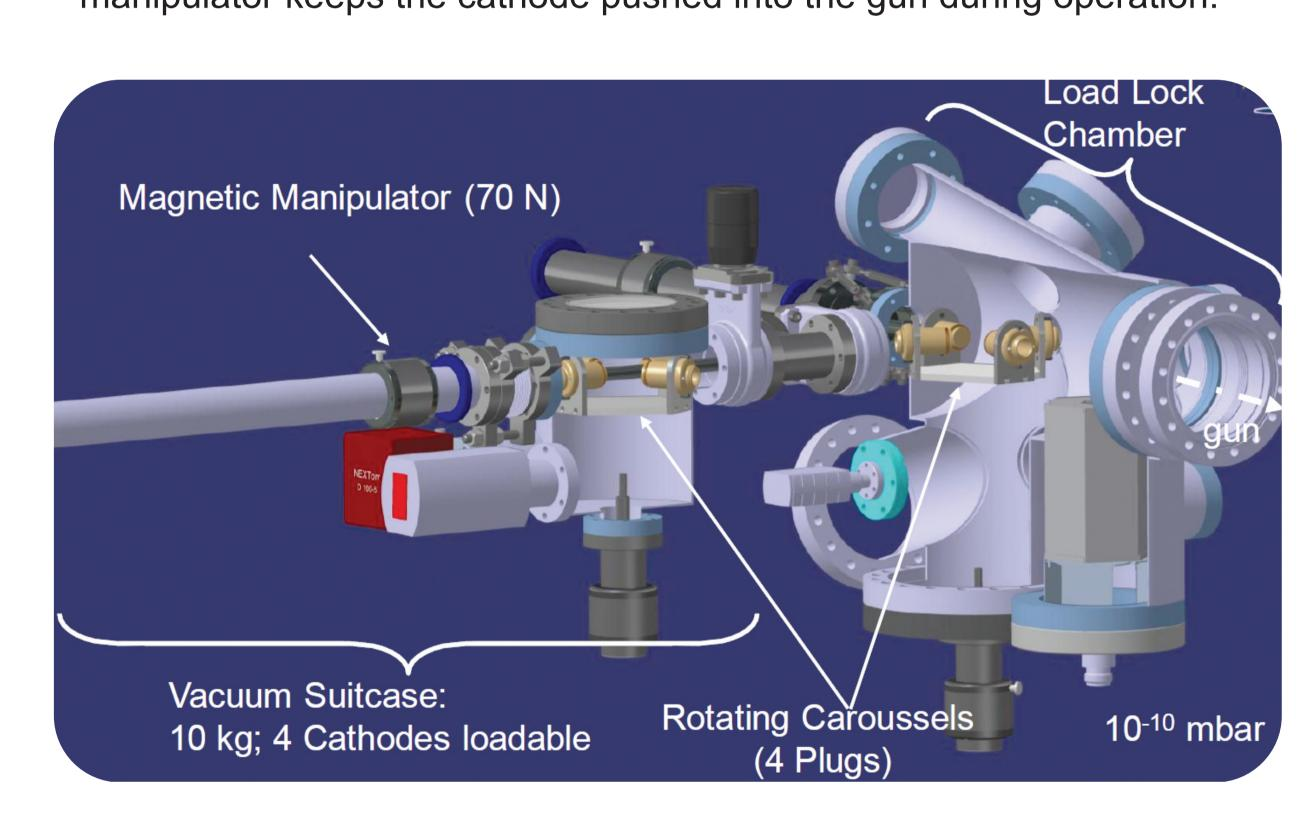
Cathode surface cleaning is done in the preparation chamber. The most effective way to remove surface contaminants is to heat up the cathode plug for several hours. The preparation chamber is equipped with a heating rod which can be directly inserted into the back of the cathode plug. Thanks to the vacuum suitcase, the cathode is protected from exposure to atmosphere. Therefore preparation processes such as Dicaesium Telluride vapor deposition can be included (see image below right).
