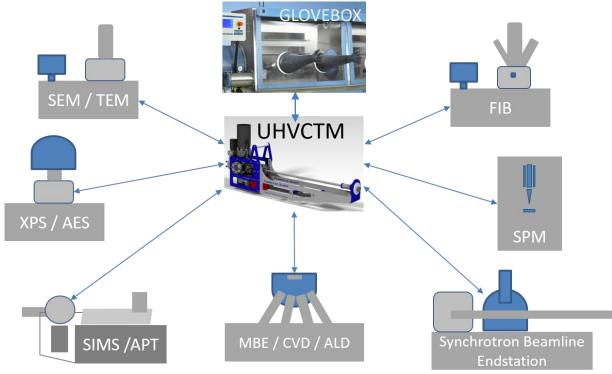
The Ferrovac UHVCTM allows for transfer of specimens under ultrahigh vacuum and cryogenic conditions between independent instruments. A glovebox for sample preparation can be of paramount importance when sample preparation under inert gas atmosphere and cryo conditions are needed.
