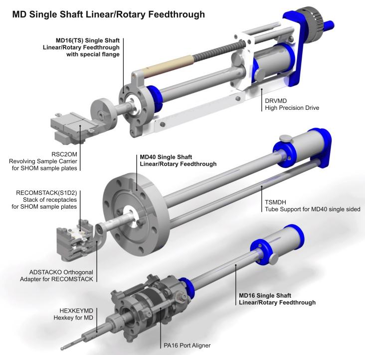
Single shaft linear/rotary feedthroughs can serve for carrying a movable sample storage platform or a stack of receptacles. If used with a port aligner and one of our key adapters, they may also be used to tighten a screw or engage a sample locking mechanism at a specific position.
