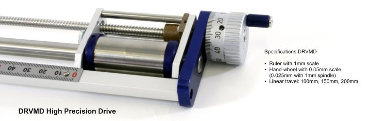
The MD16(TS) miniature and MD40 linear rotary feedthrough can be equipped with a high precision spindle drive. With a 2mm pitched spindle, a readout of 0.05mm is possible. Alternatively, a 1mm pitched spindle provides an even higher resolution.
