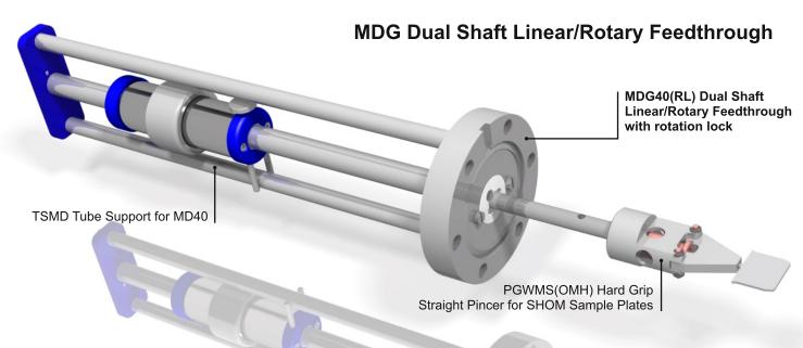
Dual shaft linear/rotary feedthroughs can be equipped with one of our pincer grips. The fine adjustable magnetic coupling allows a precise control of their opening and closing by turning a knurled screw.
