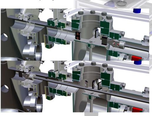
A key feature of the VSNH40 is the option to install a revolving storage platform for multiple samples. This allows the user not only to transport just one sample at a time, but also to store a larger number of samples under true UHV conditions and to exchange several samples at once.
