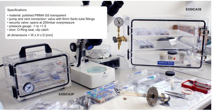
After pumpdown with a membrane pump, the exsiccator holds a base pressure of approximately 25mbar over a period of several months. A pressure meter roughly indicates the vacuum level. The box can be filled with dry Nitrogen or Argon if desired. An overpressure valve is provided for safety reasons. Standard, portable and extrawide versions of the vacuum desiccator are available.
