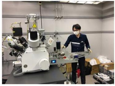
The docking kit attaches to the L-port dedicated for 3rd party components of the DualBeam™ instrument. 3 different configurations are available:
